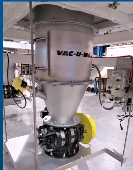
Rotary Valve Discharge on a BBU
